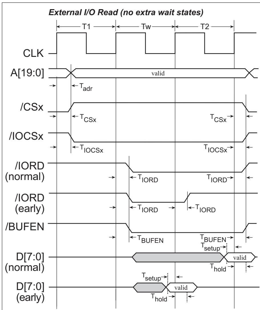
**Figure 27-3. I/O Read Cycles—No Extra Wait States**
