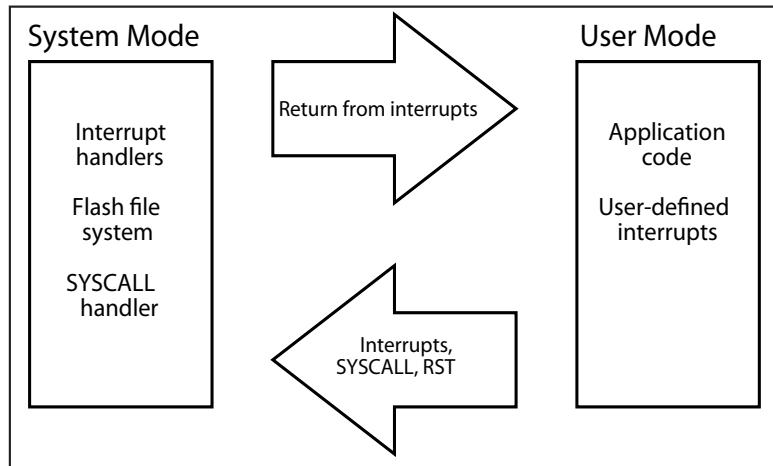
*Figure 26-3. System/User Mode Setup for Operating System*
