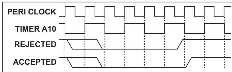
The Quadrature Decoder generates an interrupt when the counter increments from 0xFF (0x3FF in 10-bit mode) to 0x00, or when the counter decrements from 0x00 to 0xFF (0x3FF in 10-bit mode). The timing for the interrupt is shown below. Note that the status bits in the QDCSR are set coincident with the interrupt, and the interrupt and status bits are cleared by reading the QDCSR.
