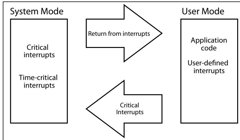
**Figure 26-2. System/User Mode Setup for Mixed Operation**
