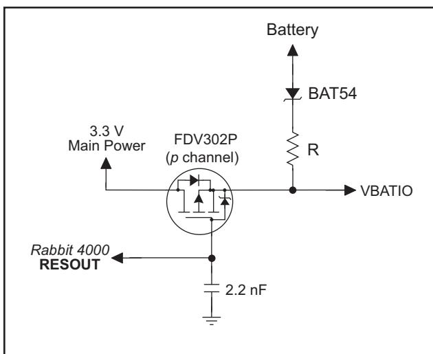
**Figure 27-8. Switching Circuit for VBATO Pin**
