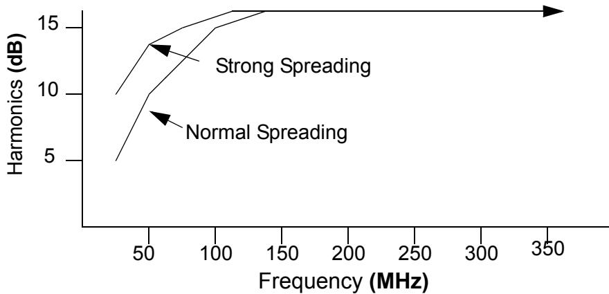
**Figure 2-2. Peak Spectral Amplitude Reduction by Spectrum Spreader**
