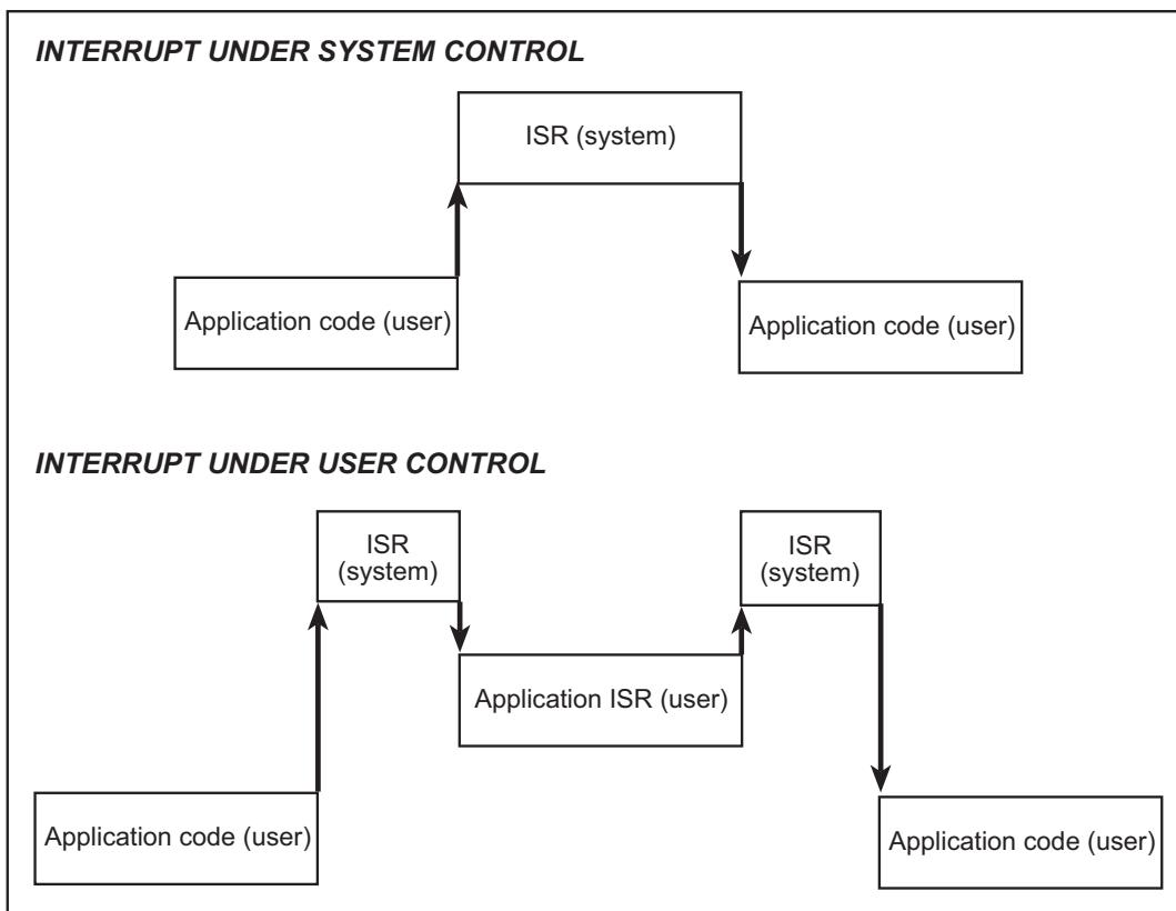
Figure 26-4. Interrupt Handing in the System/User Mode
