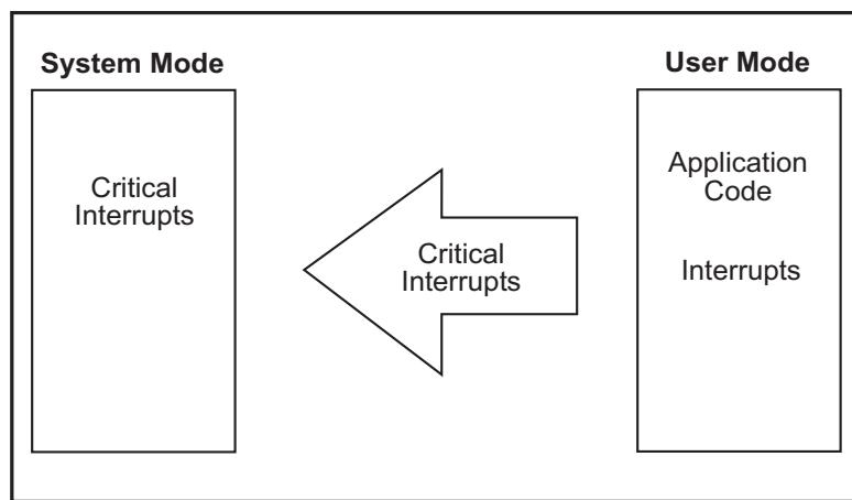
*Figure 26-1. System/User Mode Setup for Memory Protection Only*
