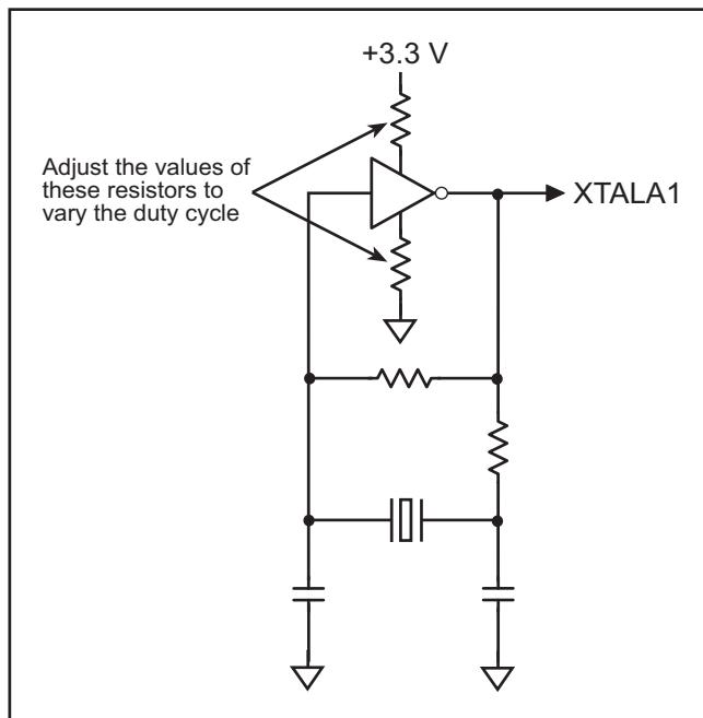
*Figure 27-5. External Oscillator Buffer*
