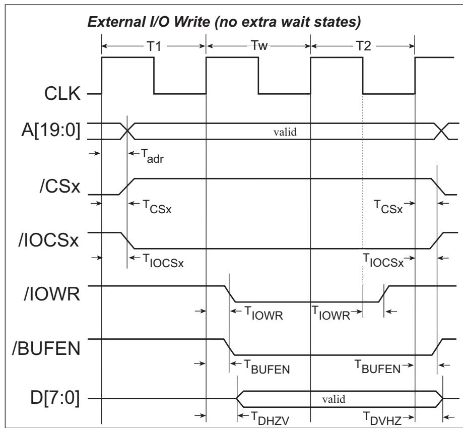
**Figure 27-4. I/O Write Cycles—No Extra Wait States**
