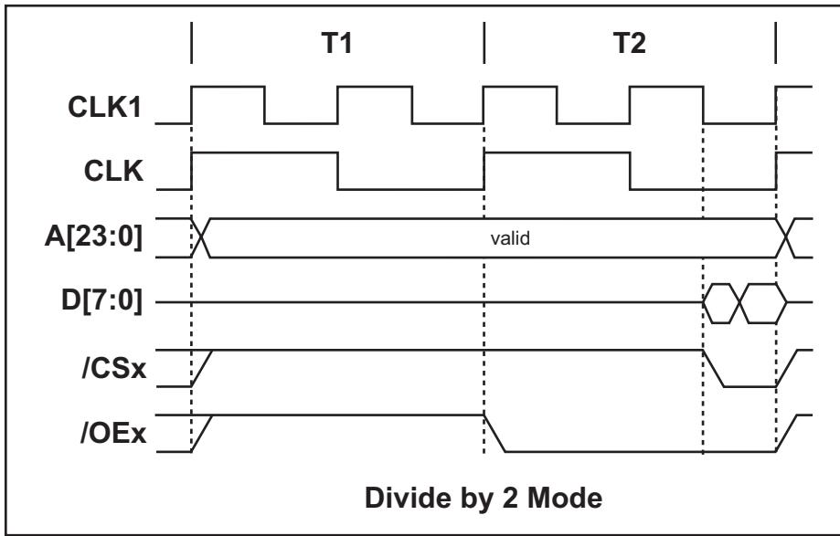
When the processor is running off the 32 kHz clock, the short chip select option will produce chip select signal that is the width of a single 32 kHz clock (30.5 microseconds); otherwise the timing is identical to the short chip select options based off the main oscillator. Read strobe figures are shown below.
