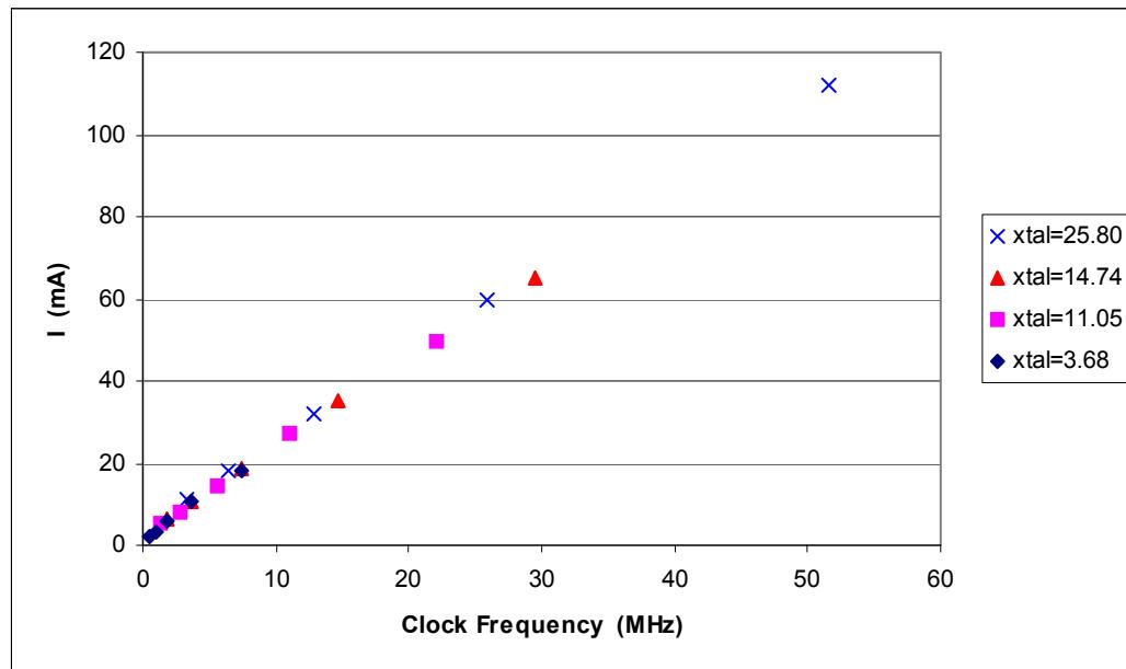
Figure 25-1. Rabbit 3000 System Current vs. Frequency at 3.3 V
