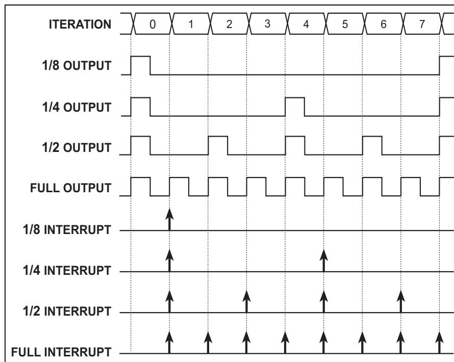
*Figure B-21. PWM Interrupt and Output Timing*
