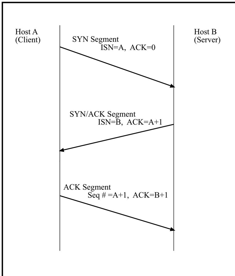
The sequence number is used to ensure the data is reassembled in the proper order before being passed to an application protocol.
