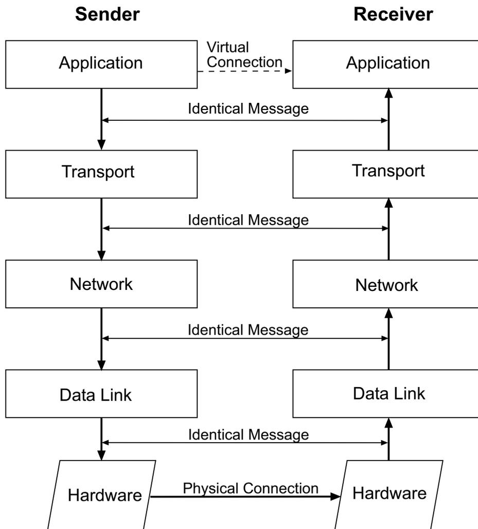
Each host or router in the internet must run a protocol stack. The details of the underlying physical connections are hidden by the software. The sending software at each layer communicates with the corresponding layer at the receiving side through information stored in headers. Each layer adds its header to the front of the message from the next higher layer. The header is removed by the corresponding layer on the receiving side.
